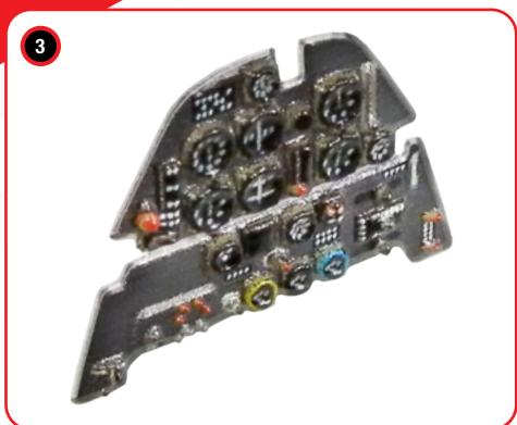
The panels come completely painted, with raised and recessed details as well as a lifelike glass effect on the instruments, they only need to be glued in place.
