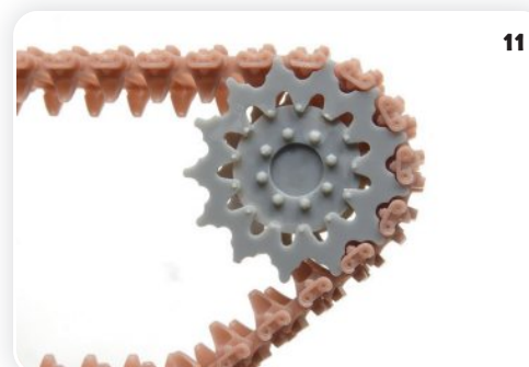
11 - Once the inner end connectors have been installed, check the fit around the drive sprocket . As shown here, the end connectors should engage correctly with the sprocket teeth without interference.
